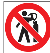
USE OF COMPRESSED-AIR TO DUST BODY PROHIBITED
